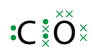
Figure 4.24 The structure of carbon monoxide if two 'ordinary' covalent bonds were formed.
