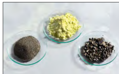
Figure 1.3 Iron (left) combines with sulfur (centre) to form iron sulfide (right).
