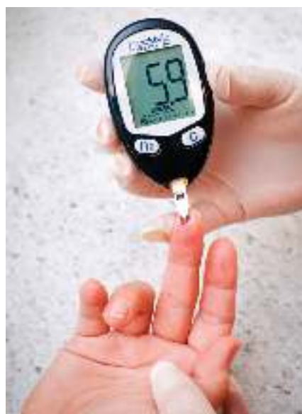
Figure 14.29: Biosensors use biological materials, such as enzymes, to measure the concentration of molecules such as glucose. This glucose biosensor is used to check the glucose concentration in a sample of blood. The meter shows a reading in the normal range.
