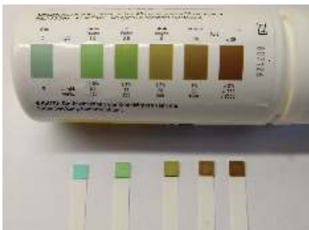
Figure 14.27: Test strips for detecting glucose in urine. After being immersed in urine the colours on the pads are compared with a colour chart provided with the test strips.
