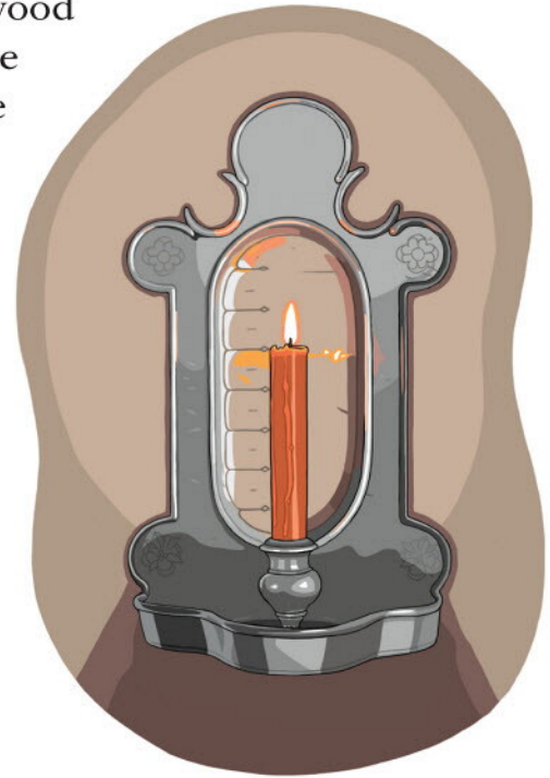
A candle divided by marks into hours functioned as a primitive clock.
